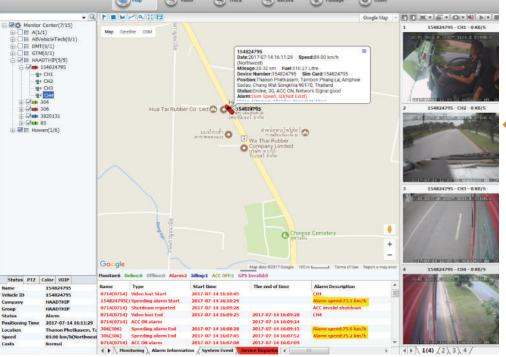
MDVR software and hardware working in tandom. A driver, side and front camera feed can be seen, as well as live tracking and incident updates
